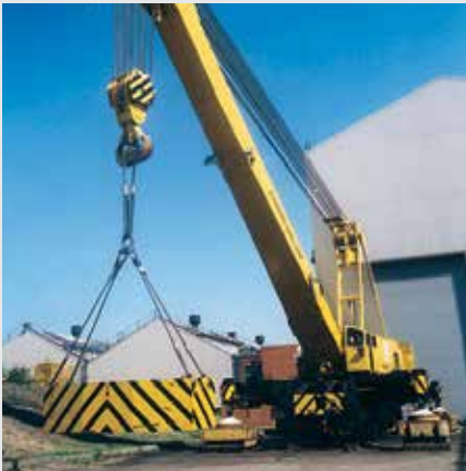
Cowans Sheldon 140 tonne rail crane.
