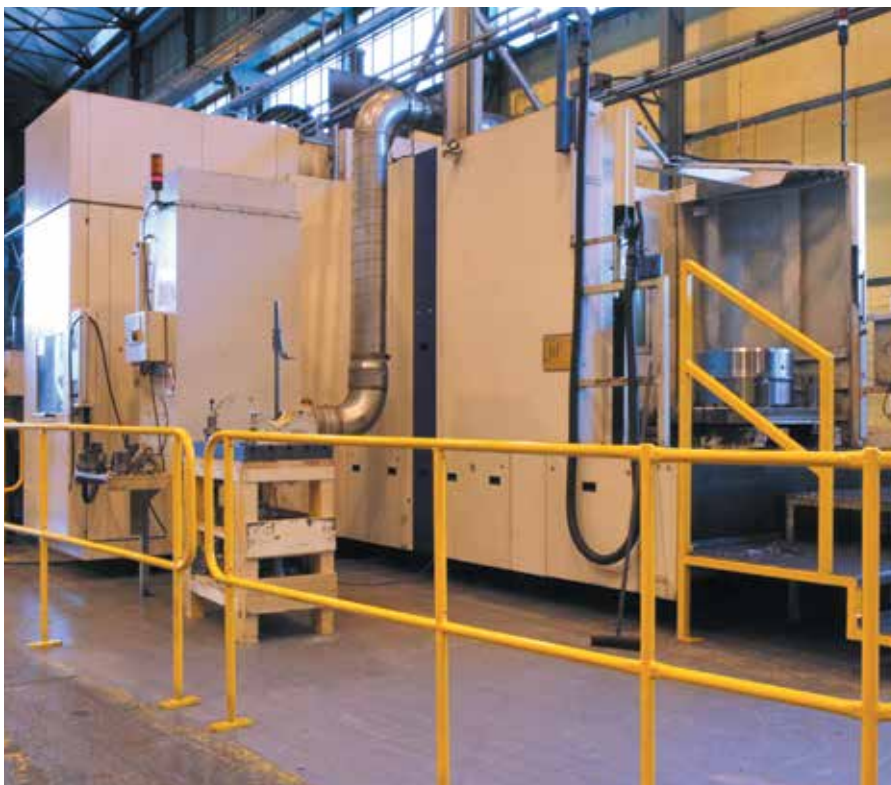
Clarke Chapman Heller 5-axis machining centre.
