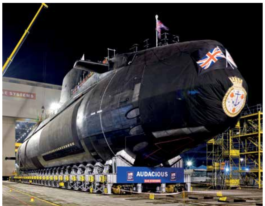
Clarke Chapman produced the transfer car system used to launch the latest Astute Class nuclear submarine, HMS Audacious.
