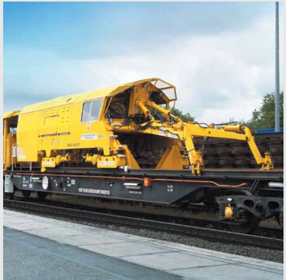
Cowans Sheldon track laying technology.
