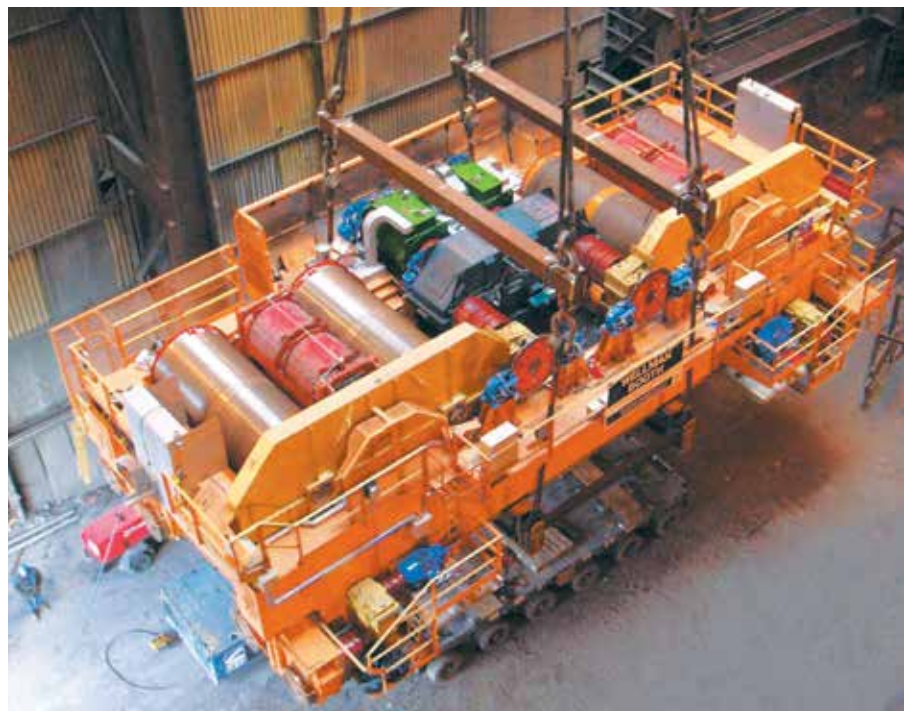
Wellman Booth 480 tonne crane main trolley unit upgrade.
