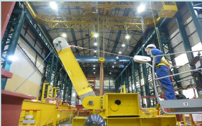
Link arms lowered to join the north and south girders
