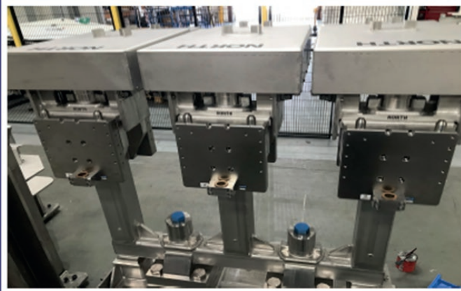
Kuka Robots Schunk Tool Adaptor Plates fitted to Tool stands – Primary and Secondary
