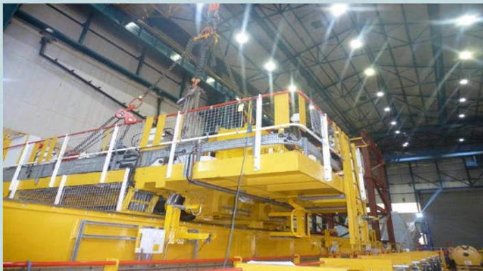
Link arms lowered to join the north and south girders
