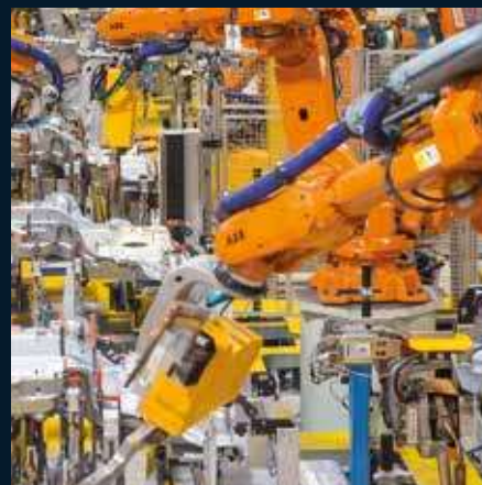
ARO 3G robotic gun technology employed at a Jaguar Land Rover plant in the UK.
