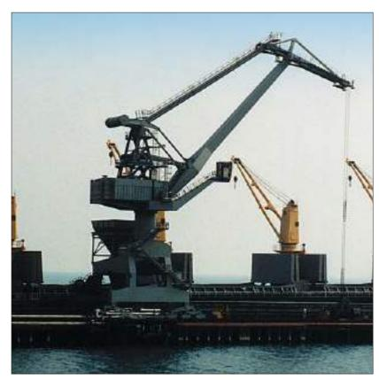
importance in bulk terminals and Stothert & Pitt select only the most reliable machinery and electrical control systems to ensure maximum availability and low cycle times. Operator's cabs are positioned to give optimum visibility both into the ship's holds and the land-side facilities.
