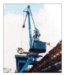
'...the ability of the crane to transfer loose bulk materials directly from ships' holds to land based moving conveyors...'
