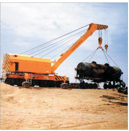
The CCS 65 – 8T, 65 tonnes at 8 metres radius capacity diesel hydraulic railway breakdown crane, two units have been delivered to Sudan Railway Corporation and one is seen recovering a tanker wagon.
