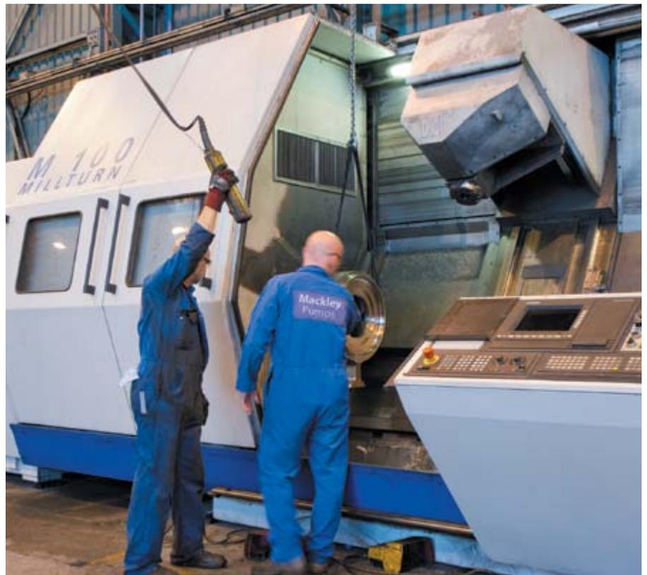
5 axis CNC mill-turn machine.
