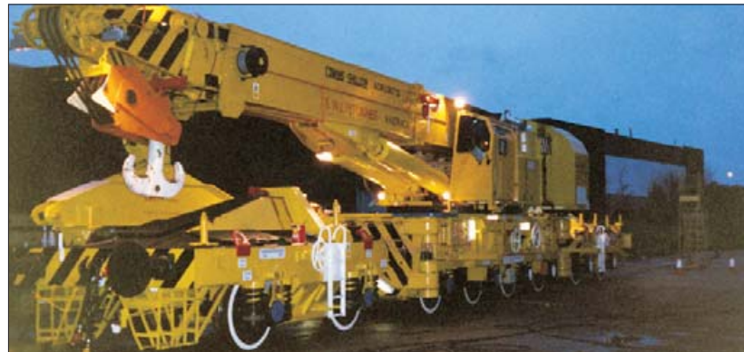
75T railway crane after refurbishment.
