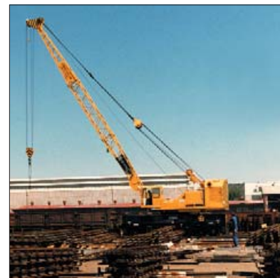
10 tonne rail crane. SAR
