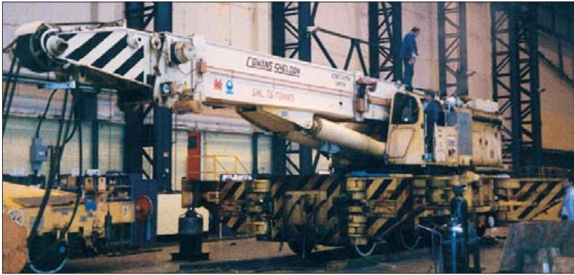
75T crane originally supplied in 1975 arrives at works for refurbishment.
