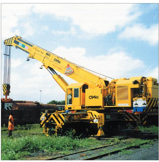
The CCS 80 – 6T, 80 tonnes at 6 metres radius capacity diesel hydraulic railway
