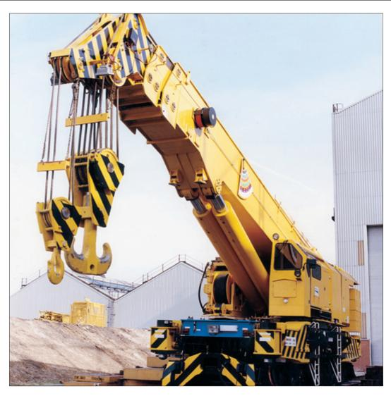
The RC 110 - 11T, 110 tonne capacity multi tasking railway recovery crane delivered to the Freight Rail division of the state Rail Authority of New South Wales in March 1995.
