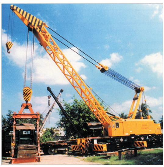
The CCS 140 – 10T, 140 tonnes at 10 metres radius capacity diesel hydraulic railway breakdown crane, ten units have
