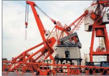
Bristol Port Authority: This crane was made safe after being hit by a ship and landing on the adjacent hopper and quayside crane.
