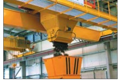
The design, manufacture and installation of a special purpose semi automatic concrete delivery crane.
