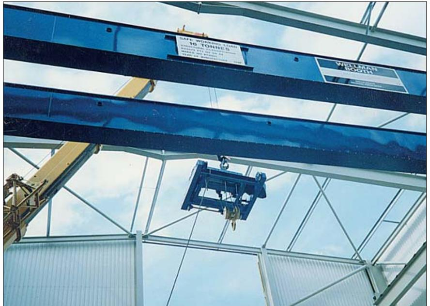
Design, manufacture and installation of 16T electric overhead travelling crane for combined heat and power facility in Derby.
