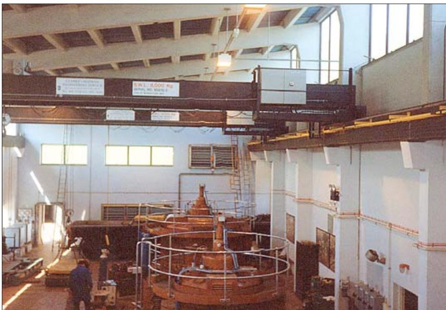
Welsh Water: Removal of two manually operated cranes and design, manufacture and installation of two 8 ton electric overhead cranes in hydro power station
