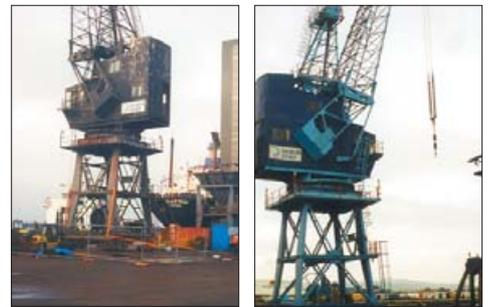
The mechanical/structural refurbishment and complete replacement of the electrical control system of two Stothert & Pitt 10 ton grabbing cranes. New drivers cabins were designed for for all round visibility and driver comfort.
