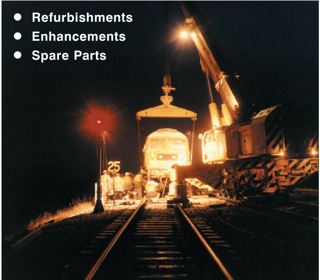
The cranes, originally supplied in the 1970's, were becoming increasingly unreliable and requiring more maintenance. The obsolescence of much of the equipment was also prohibiting spares support. A total overhaul and refurbishment has extended the service life of these cranes by another 20 years and incorporated safety modifications to bring
