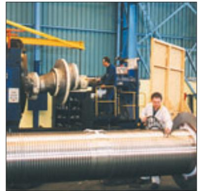
*Final inspection of crane winch drum – steel industry*
