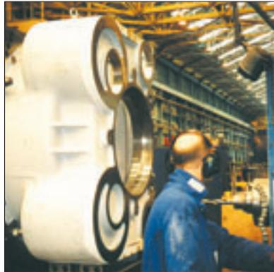
Machining of a diesel engine casting
