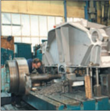
Line boring a winch frame fabrication
