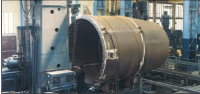
Machining of a crane pedestal fabrication – offshore industry
